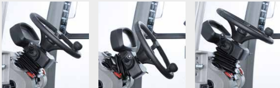
Steering wheel: Individually adjustable in height and angle – the display swivels with
