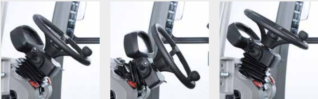
Steering wheel: Individually adjustable in height and angle – the dash board swivels with the steering wheel column
