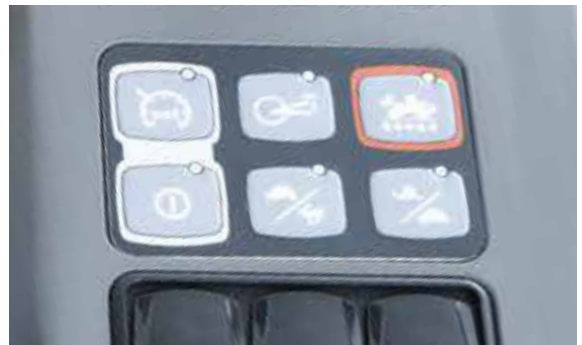
Controller: Variable key fields for driving and working modes
